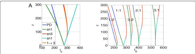
Figure 1 (A) Various bifurcations shown in 1:1 phase locked solutions. PD: Period-doubling; sn1: saddle-node in switching manifold once; sn3: saddle-node in switching manifold three times,  $1 \rightarrow 3$ , transition from sn1 to sn3. (B) Frequency mode locked solutions shown in the marked Arnol'd tongue structure.
